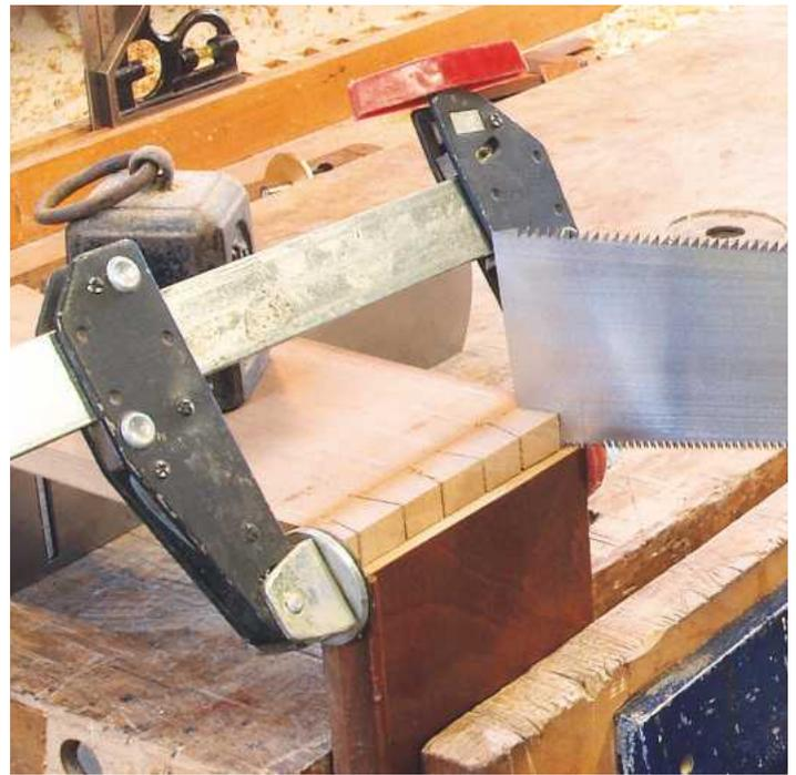
▲ Pic.7 Marking the saw cuts onto the pinboard in the old-fashioned way
